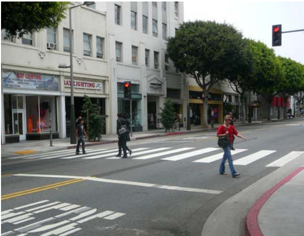
High-Visibility Crosswalks and Advanced Stop Lines at a Signalized Mid-Block Crossing
